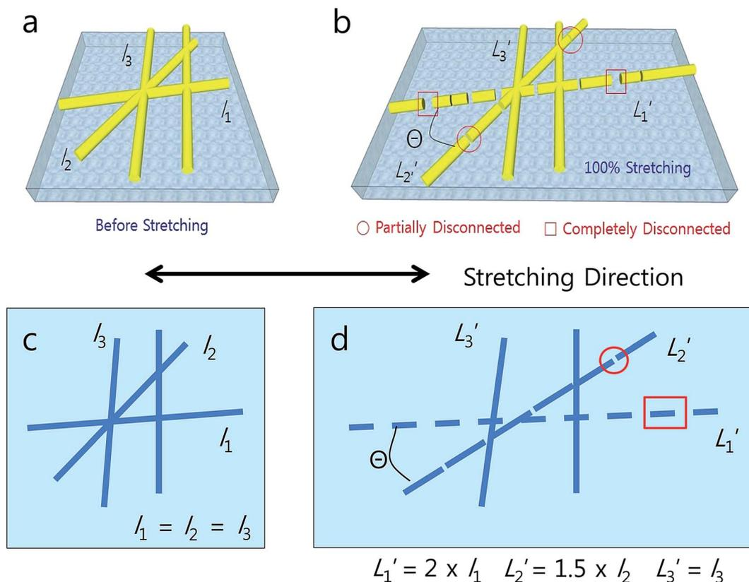
**Fig. 6** (a and b) Schematic illustrations of the evolution of the aligned electrospun fiber web under the applied strain before and after strain (100%). (c and d) Changes of the stretching length of the aligned electrospun fiber web under the applied strain before and after strain (100%).
