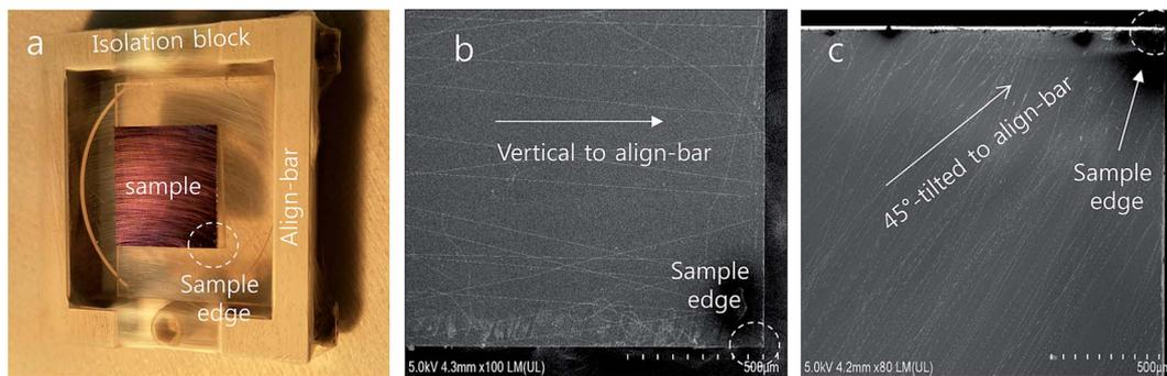
Fig. 7 (a) Photographic image of rectangular alignment jig where the substrate was inserted between a pair of alignment bars. (b) SEM images of fibers vertically aligned to the alignment bar collected directly on the sample surface using a parallel alignment jig. (c) SEM image of 45°-tilted fibers made using a rectangular alignment jig.
