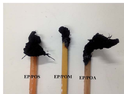
Fig. 8 Digital photos of char residue of EP/PPDA composites after LOI tests.
