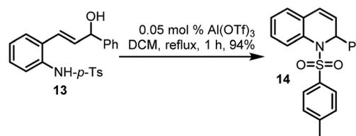
Scheme 6 Synthesis of dihydroquinoline in an Al(OTf)<sub>3</sub>-catalysed dehydrative cyclisation.
