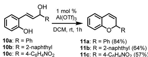
Scheme 4 Synthesis of 2*H*-chromenes in Al(OTf)<sub>3</sub>-catalysed cyclisation reactions.
