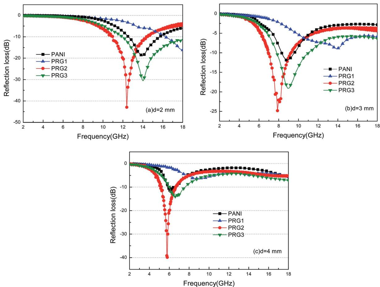
Fig. 8 The calculated reflection losses for PANI and RGO-PANI composite samples with  $d = 2$  mm (a), 3 mm (b) and 4 mm (c) in the frequency range of 2–18 GHz.
