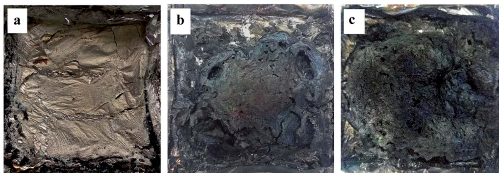
Fig. 10 Digital photos of cone calorimeter residues of (a) pristine PBT; (b) 10% AlPi/PBT; (c) 10% 1PTAC–MMT/5AlPi/PBT.
