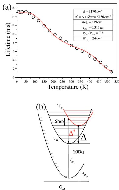
Fig. 10 (a) Decay times of the  ${}^2\text{E}$  state as a function of temperature (10–550 K) for  $\text{Ba}_5\text{AlF}_{13}:\text{Mn}^{4+}$  (0.5 mol%). (b) Energy level diagram including the ground state and the lowest excited states without spin-orbit interaction.
