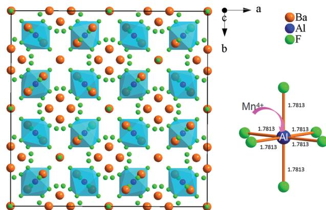
Fig. 3 Unit cell of the cubic-type  $Fd\bar{3}m$  crystal structure of  $\text{Ba}_5\text{AlF}_{13}$  projected along the  $c$  axis and coordination of the  $\text{Al}^{3+}/\text{Mn}^{4+}$  ions in this cubic-type crystal structure. Ba, F, and Al/Mn ions are represented with orange, green, and blue spheres, respectively.
