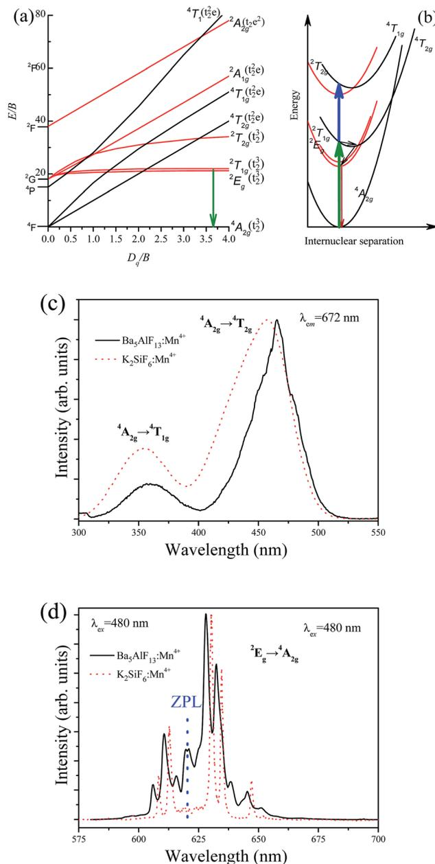
Fig. 5 (a) Tanabe–Sugano energy-level diagram for  $d^3$  ions in the octahedrally coordinated environment. (b) Configurational coordination diagram for  $\text{Mn}^{4+}$  ions in fluoride hosts. Normalized excitation spectrum (c) and emission spectrum (d) of  $\text{Ba}_5\text{AlF}_{13}:\text{Mn}^{4+}$  (0.5 mol%) compared with the well-known  $\text{K}_2\text{SiF}_6:1\% \text{Mn}^{4+}$  red phosphor.
