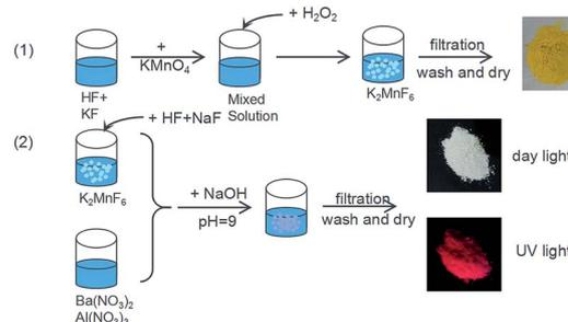
Fig. 1 Two-step synthesis of the Ba<sub>5</sub>AlF<sub>13</sub>:Mn<sup>4+</sup> nanoparticles.
