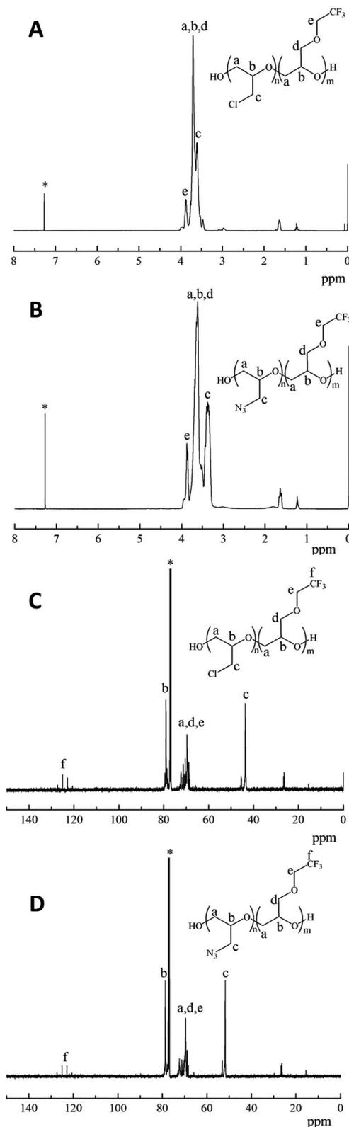
Fig. 2 <sup>1</sup>H NMR spectra of (A) poly(TFEE-*r*-ECH), (B) poly(TFEE-*r*-GA), <sup>13</sup>C NMR spectra of (C) poly(TFEE-*r*-ECH), (D) poly(TFEE-*r*-GA).
