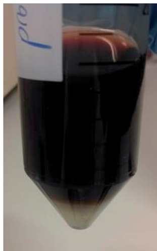
Fig. 6 \text{PbSO}_4 precipitate obtained by addition of \text{H}_2\text{SO}_4 to the acetic acid leachate of the matte.
