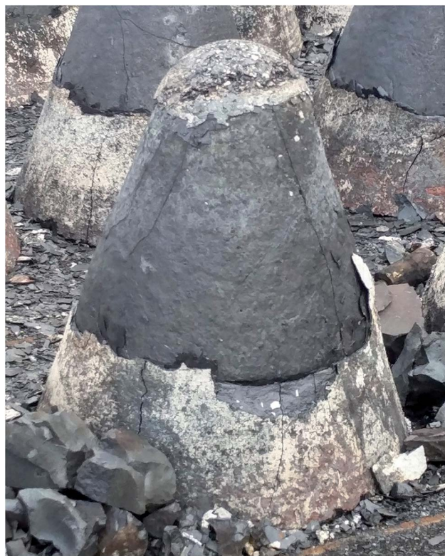
Fig. 1 Inverted slag pots, showing the slag at the bottom (light grey) and the matte (dark grey) at the top.
