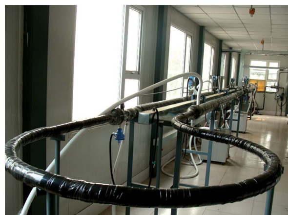
Fig. 1 (Left) Schematic diagram of the high pressure hydrate flow loop; (Right) photograph of the flow loop test section.
