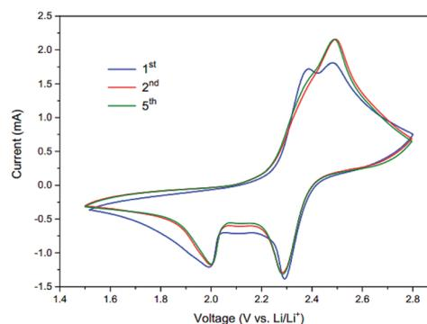
Fig. 5 Cycle voltammograms of the PVP-S/GA cathode at  $0.1 \text{ mV s}^{-1}$  from 1.6 to 2.8 V vs.  $\text{Li/Li}^+$ .
