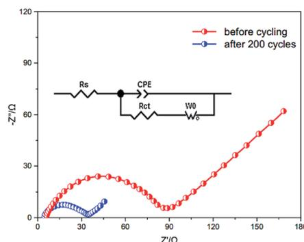
Fig. 8 Electrochemical impedance spectra of the PVP-S/GA cathode and the equivalent circuit model.
