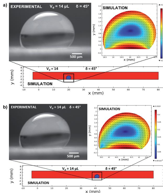
Fig. 12 Droplet location on an inclined surface and velocity field predicted from the simulations. (a) Velocity field inside the droplet located 20 mm on the inclined surface. (b) Velocity field ( $\text{m s}^{-1}$ ) inside the droplet located 40 mm on the inclined surface.
