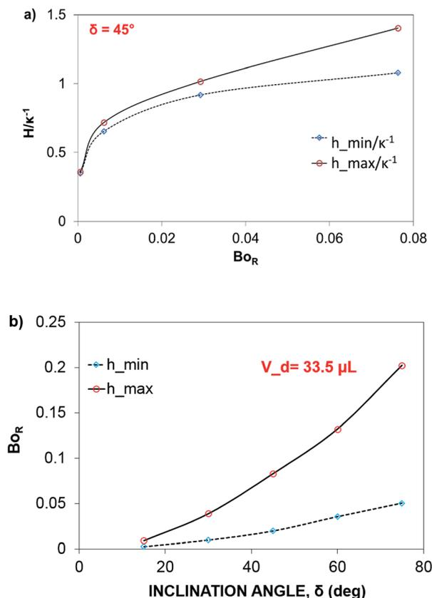
Fig. 11 Maximum and minimum droplet heights during droplet rolling on a hydrophobic surface.  $\kappa$  is the capillary length. (a) Normalized maximum and minimum droplet heights versus rotational Bond number for a droplet volume  $V_d = 33.5 \mu\text{L}$ . (b) Rotational Bond number at maximum and minimum droplet heights versus surface inclination angle.
