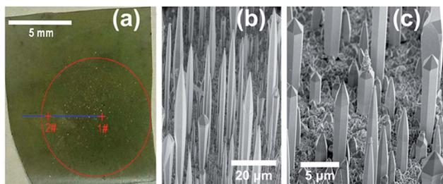
Fig. 4 (a) The optical photograph and the SEM images at point (b) 1#, (c) 2# of sample B2.
