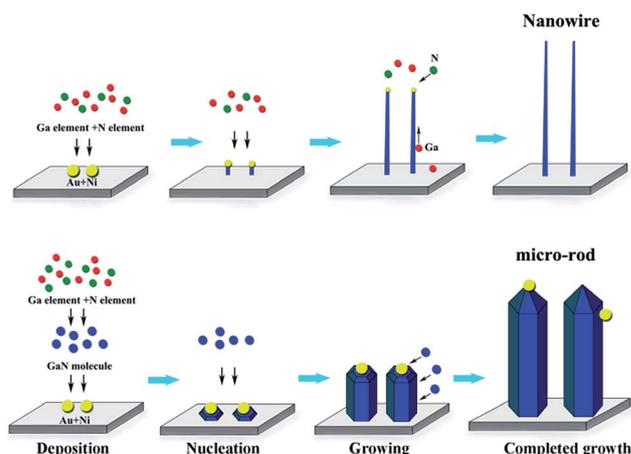
Fig. 6 The growth mechanism schematic of nanowires and micro-rods.
