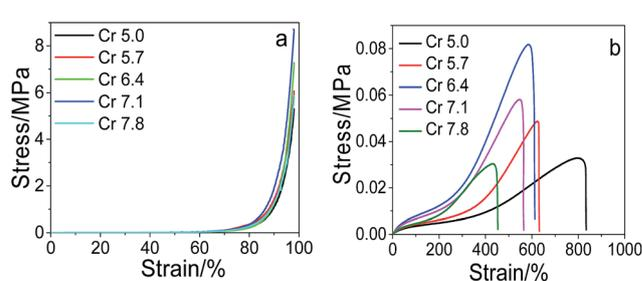
Fig. 3 Compressive (a) and tensile (b) stress–strain curves of the prepared hydrogels with varying crosslinkers (at fixed SC of 20 wt%, MACS of 20 wt%, KPS of 0.22 mol%).
