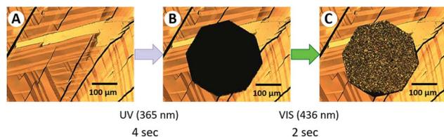
Fig. 2 Optical micrographs of **Azo** films prepared on glass substrates. (A) As prepared, (B) UV irradiated at 365 nm for 4 s in the octagonal area; and (C) exposure to visible light at 436 nm for 2 s following UV irradiation.
