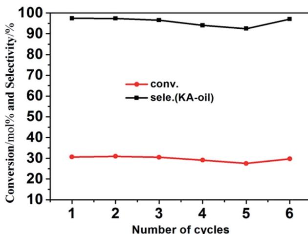
Fig. 7 Catalytic performance of the obtained 2% Mn-ZSM-5 (P<sub>3</sub>) during different cycles.
