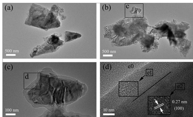
Fig. 2 TEM images of MoS<sub>2</sub> and MoS<sub>2</sub>-PDA-MGA: (a) MoS<sub>2</sub>, (b-d) MoS<sub>2</sub>-PDA-MGA.
