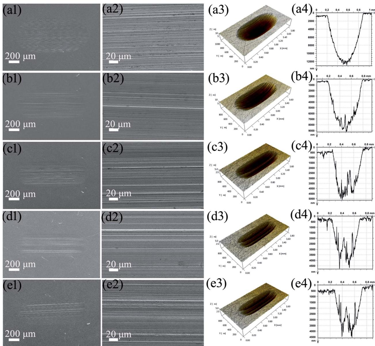
Fig. 10 SEM images and 3D optical microscopic images of the worn scar surfaces lubricated by PAG oil ((a1–a4)) and with different concentrations (0.3 wt% (b1–b4), 0.5 wt% (c1–c4), 0.7 wt% (d1–d4), 0.9 wt% (e1–e4)) of MoS<sub>2</sub>-PDA-MGA under a load of 100 N (temperature, 150 °C; stroke, 1 mm; frequency, 25 Hz).
