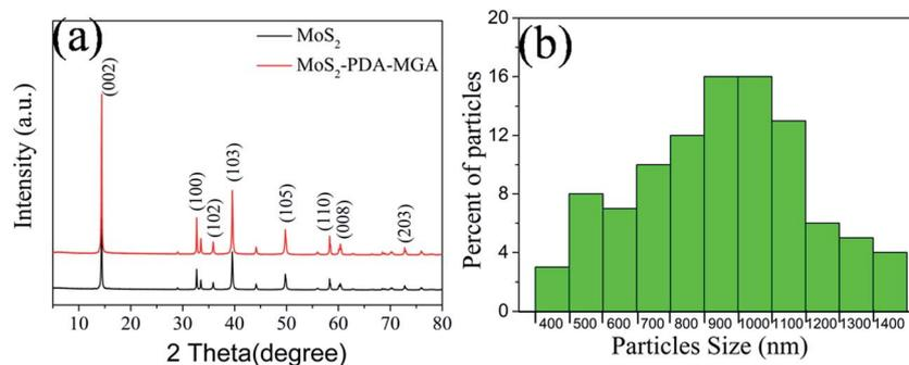
Fig. 1 XRD patterns and size distribution of MoS<sub>2</sub>-PDA-MGA.
