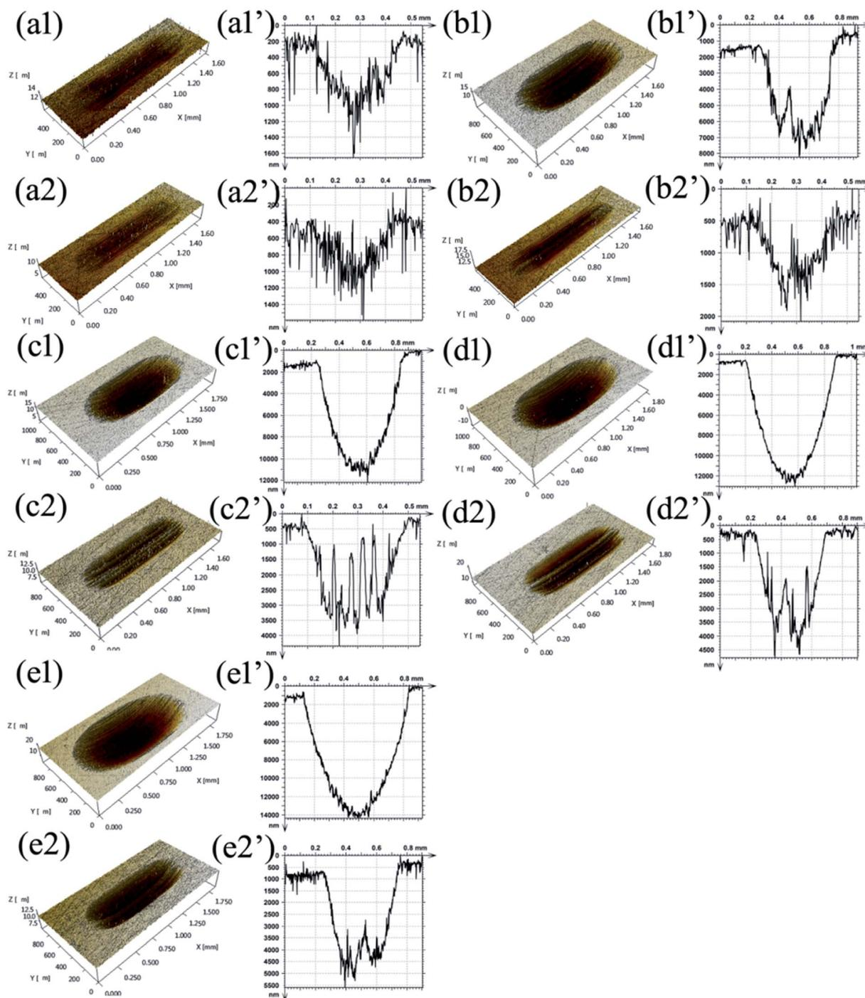
Fig. 11 3D optical microscopic images of wear scars lubricated by PAG ((a1), (a1'), (b1), (b1'), (c1), (c1'), (d1), (d1'), (e1), (e1')) and PAG containing 0.7 wt% MoS<sub>2</sub>-PDA-MGA ((a2), (a2'), (b2), (b2'), (c2), (c2'), (d2), (d2'), (e2), (e2')) under 100 N at various temperatures: (a1), (a1'), (a2), (a2') at 50 °C; (b1), (b1'), (b2), (b2') at 90 °C; (c1), (c1'), (c2), (c2') at 130 °C; (d1), (d1'), (d2), (d2') at 150 °C; (e1), (e1'), (e2), (e2') at 170 °C.
