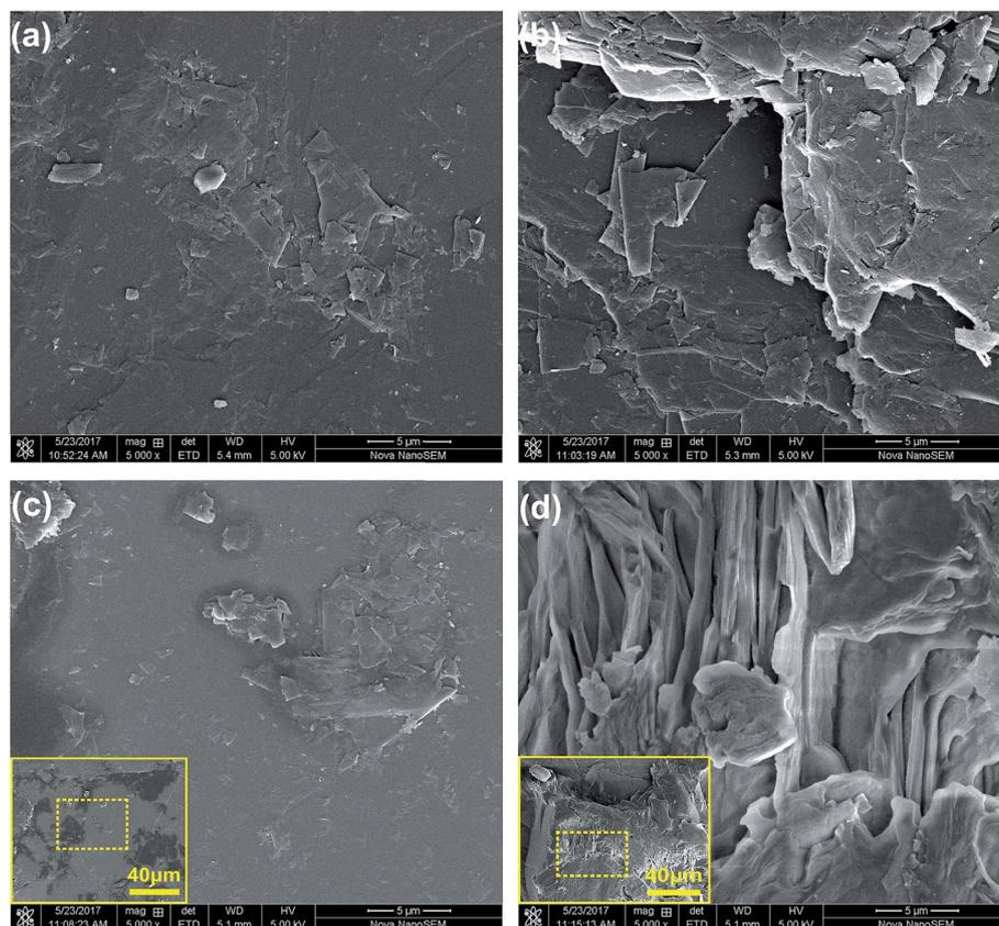
Fig. 2 SEM images of (a) FG<sub>r</sub>, (b) FG<sub>3</sub>, (c) SA/FG<sub>r</sub>, and (d) SA/FG<sub>3</sub>.
