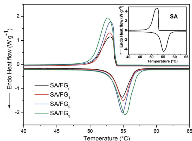
Fig. 4 DSC curves of SA and SA/FG<sub>r</sub>, SA/FG<sub>1</sub>, SA/FG<sub>2</sub>, and SA/FG<sub>3</sub> composites.
