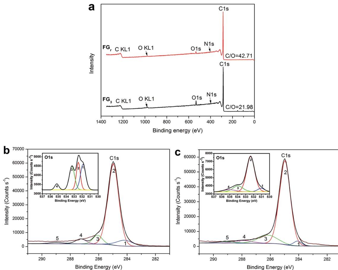
Fig. 7 (a) Full XPS spectra of the  $FG_r$  and  $FG_3$ ; C1s and O1s XPS spectra: (b)  $FG_r$ , and (c)  $FG_3$ .
