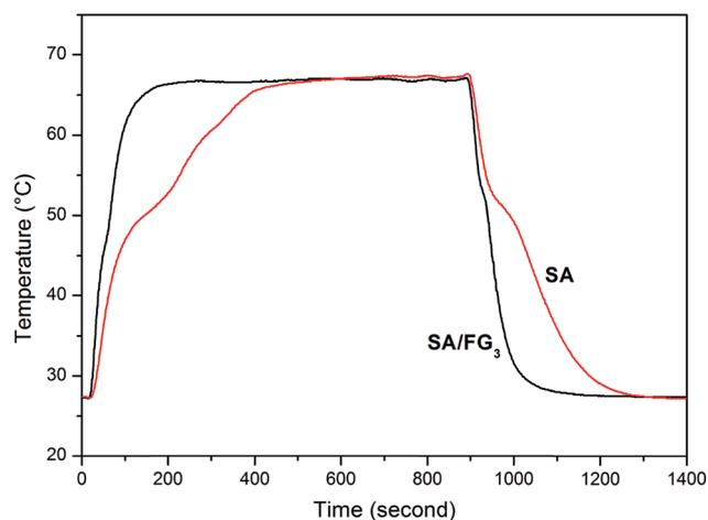
Fig. 6 Thermal storage and release performance (a) a test set-up; (b) curves of SA and SA/FG<sub>3</sub>.
