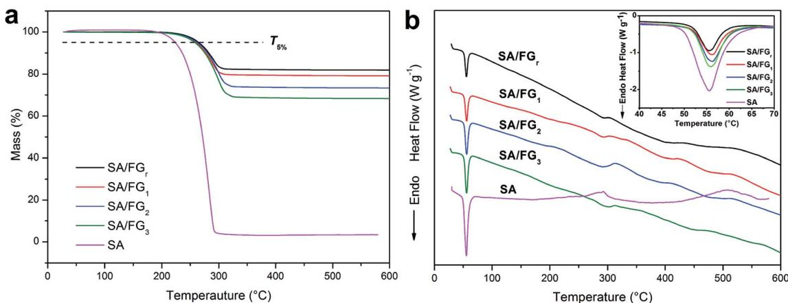
Fig. 3 TG (a) – DSC (b) of SA and SA/FG<sub>r</sub>, SA/FG<sub>1</sub>, SA/FG<sub>2</sub>, and SA/FG<sub>3</sub> composites.
