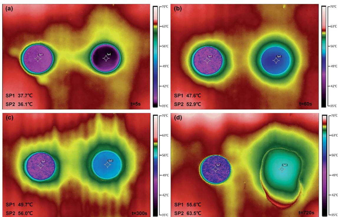
Fig. 9 Thermal images of SA/FG<sub>3</sub> (SP1) and pure SA (SP2) tableting rounds heated at different times: (a)  $t = 5$  s; (b)  $t = 60$  s; (c)  $t = 300$  s; (d)  $t = 720$  s.
