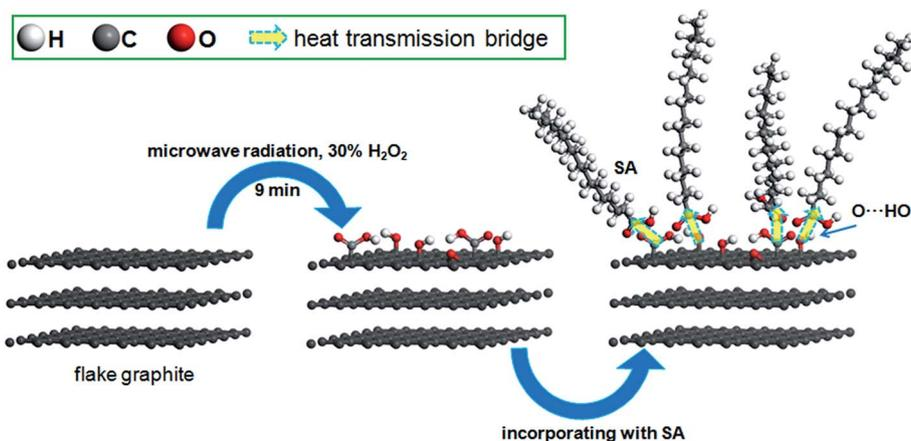
Fig. 8 Illustration of the mechanism of enhanced performance of SA/FG<sub>3</sub>.
