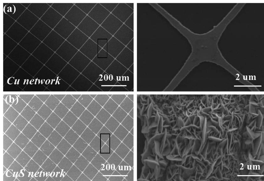
Fig. 2 (a) SEM image of the Cu networks and magnified meshes. (b) SEM images of the flower-like CuS generated on the Cu meshes.
