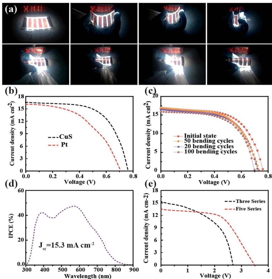
Fig. 4 (a) Photographs showing the mechanical flexibility of the ultrathin and light tandem DSSC. (b)  $J$ - $V$  curves of the two different DSSCs based on CuS and Pt CEs. (c)  $J$ - $V$  curves of the flexible single DSSC with different bending cycles. (d) Incident photo-to-current conversion efficiency (IPCE) curve of the DSSC. (e)  $J$ - $V$  curves of several DSSCs in a tandem configuration.
