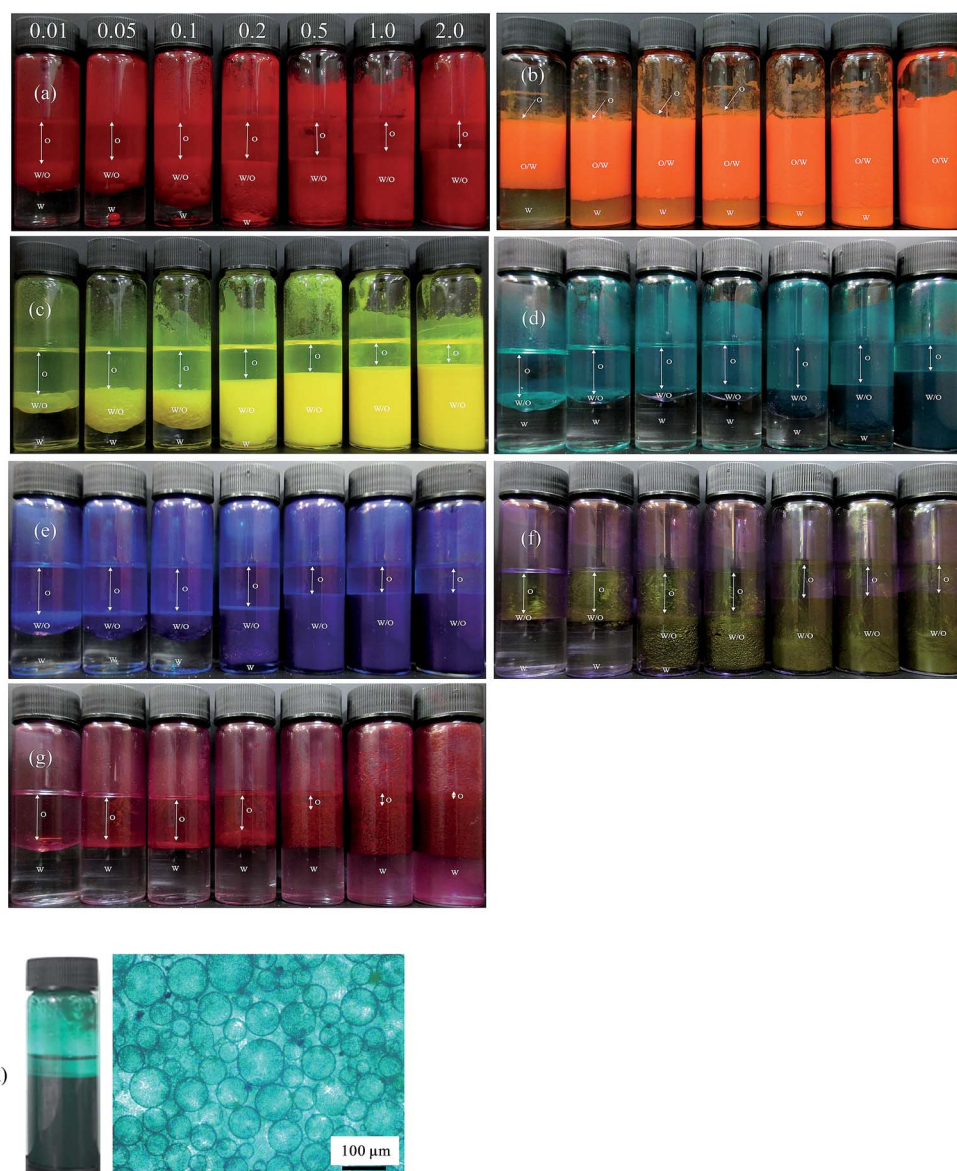
Fig. 5 Photographs of emulsions after 1 month prepared at different particle concentrations (given in wt%) for the seven pigments with \phi_w = 0.5 : (a) PR, (b) PO, (c) PY, (d) PG, (e) PB, (f) PI, (g) PV. Emulsions are w/o except those of PO which are o/w. In (h), w/o emulsion and microscope image of the mixture containing 0.5 wt% each of PY and PB.
