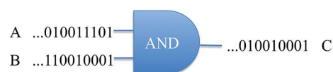
Scheme 1 A microscopic view of an AND between two molecules implemented by the progress of a bimolecular event.
