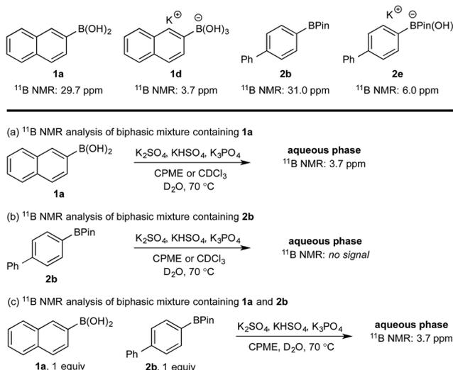
Scheme 4 <sup>11</sup>B NMR analysis of mono- and diboron systems of **1a** and **2b** under representative biphasic conditions.
