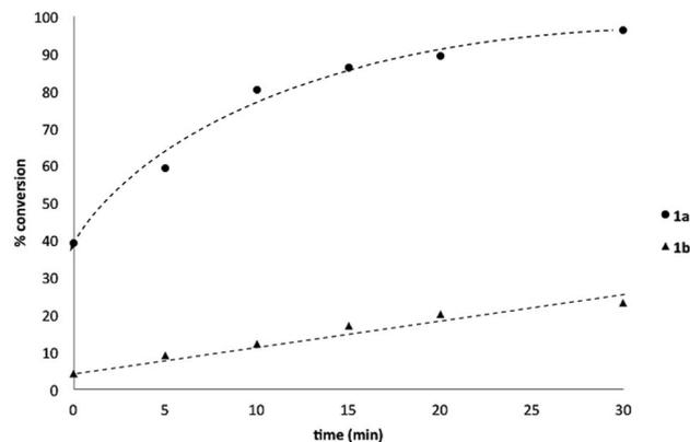
Chart 1 Oxidation of **1a** and **1b** using Oxone® under biphasic reaction conditions (THF/H<sub>2</sub>O) over 30 min at 350 rpm (*vide infra*). Determined by HPLC using an internal standard, see ESI.†§
