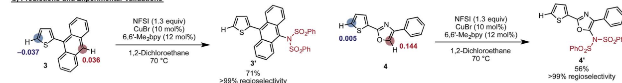
Fig. 17 Validation of a model to predict the site of C–H imidation based on the calculated Hirshfeld charges (shown in red and blue) on the DFT-optimized radical cation structure of each substrate. The experimentally imidated site is indicated by a red sphere and the site with the highest positive charge is indicated with red numbers. Other possible sites for imidation are indicated with blue spheres. Using this model, regioselectivity predictions were made for new substrates, 3 and 4. The predictions for these substrates were then validated experimentally producing the predicted product with >99% selectivity.
