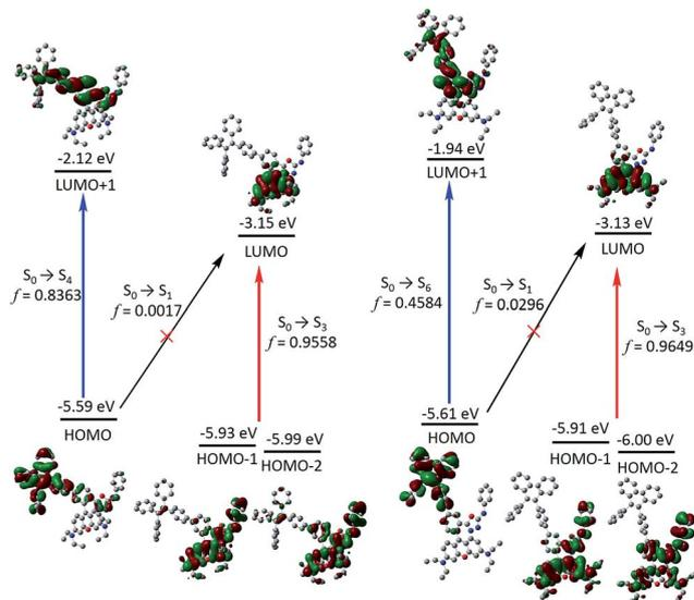
Fig. 3 Time dependent B3LYP/6-31G(d) calculated frontier molecular orbitals, energy levels, selected electronic transitions and oscillator strengths of ***p*-TPE-RNO** (left) and ***m*-TPE-RNO** (right). Note that the electron distribution and energy levels of the HOMO-1 and the HOMO-2 in each molecule are very similar. Hydrogen atoms are omitted for clarity.
