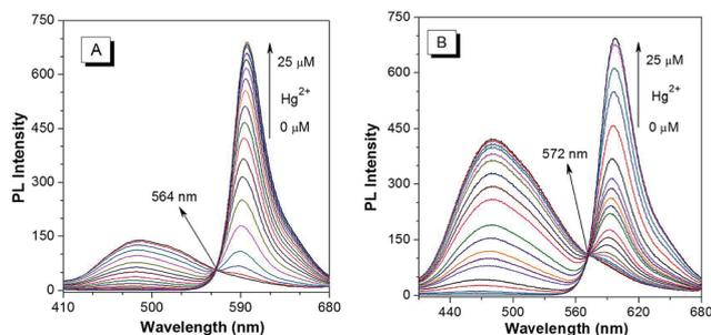
Fig. 4 PL spectra of 10  $\mu M$  (A) *p*-TPE-RNS and (B) *m*-TPE-RNS in a  $CH_3CN$ /water mixture at 60% water fraction in the presence of different amounts of  $Hg^{2+}$ . Excitation wavelength: 355 nm.
