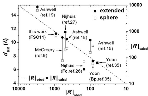
**Fig. 6** A comparison of the observed and predicted magnitudes of rectification  $|R|$  at  $\pm 1$  V based on the volume of the  $\pi$ -system confined to the head-group for FSC11 and other systems from the literatures following the methodology of ref. 35. The experimental value of  $|R|$  for FSC11 is the maximum value observed only in a few hero junctions. The two different methods of calculating volume give very similar values for FSC11 because of its spherical geometry.
