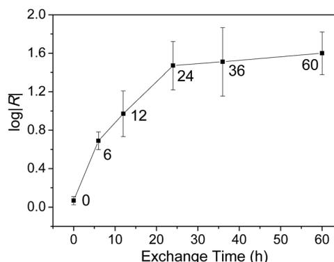
Fig. 4 A plot of  $\log|R|$  versus the time that SAMs of SC10 were exposed to solutions of FSC11 (exchange time) using EGaIn top-contacts. The magnitude of  $\log|R|$  increases gradually, saturating above 24 h, indicating the nearly complete FSC11 SAM was achieved after 24 h. The values of  $\log|R|$  and the error bars are the mean and standard deviation from Gaussian fits to histograms of  $R$  for each value of  $V$ .
