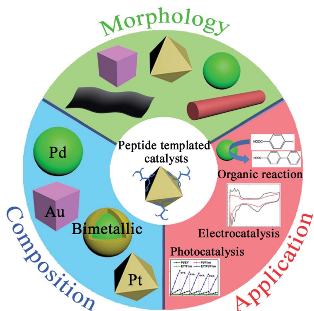
Fig. 1 Characteristics of peptide-templated noble metal catalysts, including morphologies, compositions, and applications.
