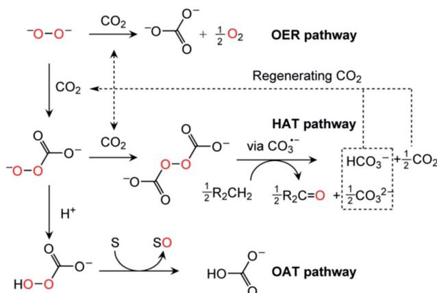
**Fig. 6** Proposed mechanistic pathways for  $\text{CO}_2$ -mediated solvent decomposition in lithium- $\text{O}_2$  batteries. OER is an "oxygen evolving reaction", HAT is a "hydrogen atom transfer" oxidative process involving hydrogen atom abstraction by carbonate radical anion, and OAT is "oxygen atom transfer" to a substrate, S.
