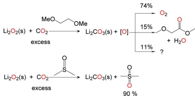
Fig. 8  $\text{CO}_2$ -mediated oxidation of organic solvents by  $\text{Li}_2\text{O}_2$ . Addition of excess  $\text{CO}_2$  to solid  $\text{Li}_2\text{O}_2$  in the organic solvent 1,2-dimethoxyethane (DME) generates an oxidizing equivalent "O", which converts to  $\text{O}_2$  (74%) and methyl methoxyacetate (15%) with the remainder unidentified. A similar reaction performed in dimethylsulfoxide (DMSO) generated dimethylsulfone ( $\text{DMSO}_2$ ) in a 90% yield.
