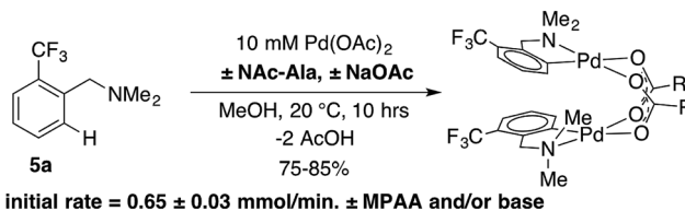
Scheme 3 MPAA and carboxylate bases showed no effect on the rate of cyclopalladation of 5a .
