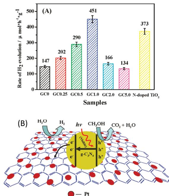
Fig. 9 (A) Comparison of the photocatalytic activities of samples with different loading amounts of graphene on g-C<sub>3</sub>N<sub>4</sub> polymers, (B) proposed mechanism for the enhanced electron transfer process of the graphene/g-C<sub>3</sub>N<sub>4</sub> polymers. Reprinted with permission from ref. 48. Copyright 2011, American Chemical Society.
