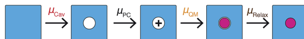
Fig. 2 Schematic of the partitioning of the single ion solvation free energies used here. The contributions are the cavity formation, point charge, quantum mechanical and hard sphere relaxation terms.
