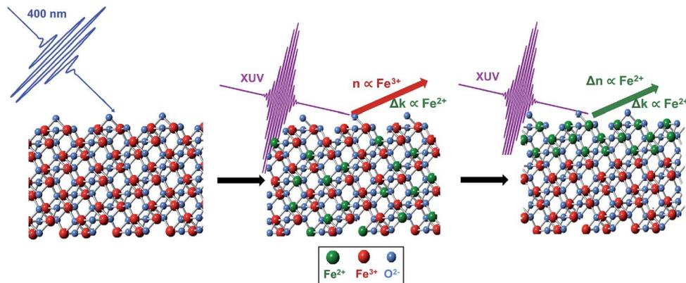
Fig. 6  $\text{Fe}_2\text{O}_3$  is initially photoexcited by a 35 fs pulse of 400 nm light. The delocalized charge carriers give rise to an RA spectrum which is composed of both  $\text{Fe}^{2+}$   $k$  and  $\text{Fe}^{3+}$   $n$  character. Over the next  $\sim 660$  fs, the excited charge carriers migrate to the surface, and the resulting RA spectra have  $\text{Fe}^{2+}$   $n$  and  $k$  character.
