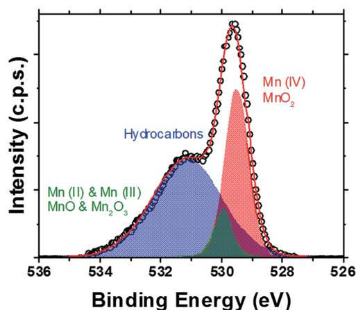
Fig. 3 XPS (high resolution scan of the peak seen in the complete survey scan, Fig. S6, ESI†) of the O 1s core level of  $\text{CoFe}_2\text{O}_4$ @ $\text{MnO}_2$  core@shell nanoparticles. Peaks represent  $\text{Mn}(\text{IV})\text{O}_2$  (red),  $\text{Mn}(\text{II})\text{O}$  and  $\text{Mn}(\text{III})_2\text{O}_3$  (green) present on the nanoparticle surfaces, as well as hydrocarbons (blue) attributed to the presence of oleic acid stabilising agents used during nanoparticle preparation.
