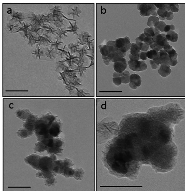
Fig. 2 Transmission electron microscope (TEM) images of (a)  $\text{MnO}_2$  nanoparticles ( $46.7 \pm 8.1$  nm), (b)  $\text{CoFe}_2\text{O}_4$  nanoparticles ( $41.0 \pm 15.1$  nm), (c) and (d)  $\text{CoFe}_2\text{O}_4@\text{MnO}_2$  core@shell nanoparticles ( $52.8 \pm 19.6$  nm). Scale bar is 100 nm.
