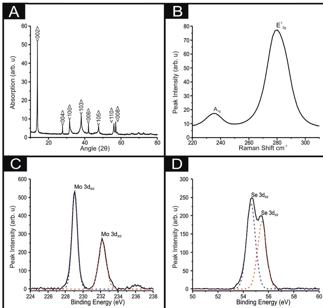
Fig. 2 Characterisation of the commercially sourced 2D-MoSe<sub>2</sub>; (A) XRD spectra of the 2D-MoSe<sub>2</sub>, (B) Raman spectra 2D-MoSe<sub>2</sub> deposited onto a silicon wafer. High-resolution XPS spectra of Mo 3d and Se 3d regions of MoSe<sub>2</sub> (C and D respectively).
