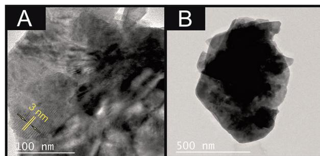
Fig. 1 TEM images of the commercially sourced 2D-MoSe<sub>2</sub>. (A) Scale bar: 100 nm, (B) scale bar: 500 nm.
