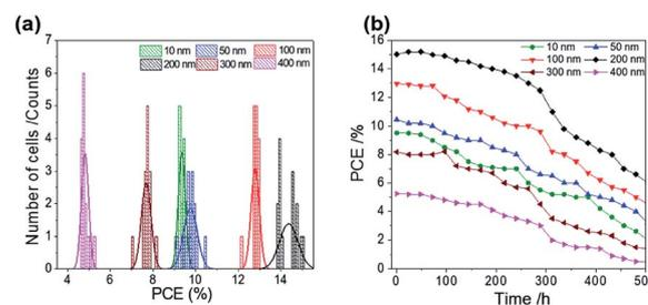
Fig. 7 (a) PCE distribution histogram; (b) PCE evolution of 15 devices stored in ambient air for varied duration/h for ALD-TiO<sub>2</sub> of thickness 10, 50, 100, 200, 300 and 400 nm, respectively, as a compact HBL.
