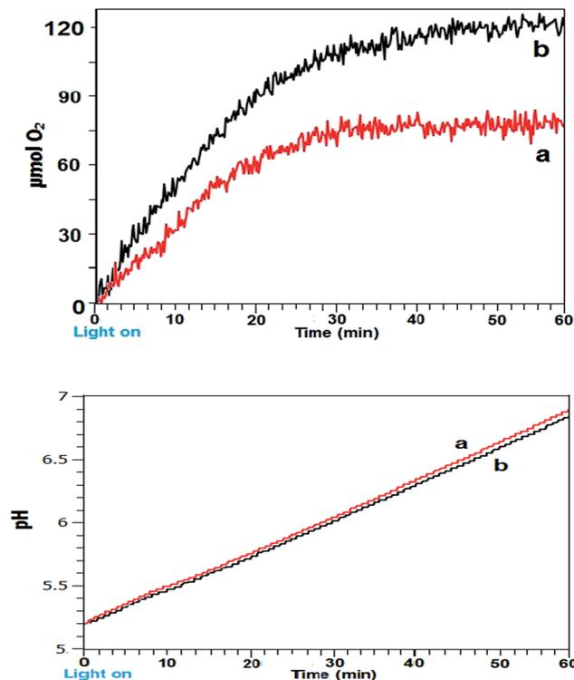
Fig. 3 (a) Graph of released  $O_2$  ( $\mu\text{mol}$ ) against time for a photocatalytic system using  $\text{Co}_3\text{O}_4$  as catalyst and light using repeated light on : off cycles (s : s) of (a) continuous; (b) 24 : 2. (b) Graph of pH change for  $\text{Co}_3\text{O}_4$  reaction systems using repeated light on : off cycles (s : s) of (a) continuous; (b) 24 : 2.
