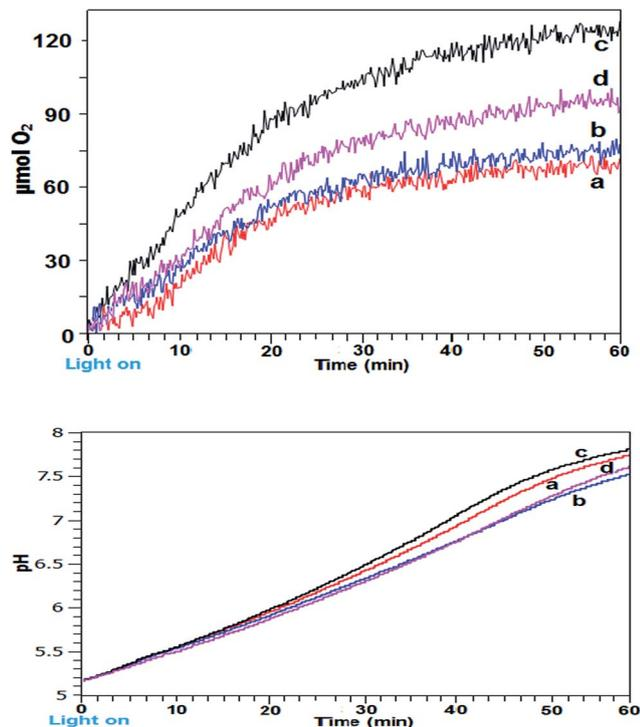
Fig. 2 (a) Graph of released  $O_2$  ( $\mu\text{mol}$ ) against time for a photocatalytic system using  $\text{CaMn}_3\text{O}_6$  as catalyst and light using repeated light on : off cycles (s : s) of (a) continuous; (b) 24 : 1.5; (c) 24 : 2; (d) 24 : 2.5. (b) Graph of pH change for  $\text{CaMn}_3\text{O}_6$  reaction systems using repeated light on : off cycles (s : s) of (a) continuous; (b) 24 : 1.5; (c) 24 : 2; (d) 24 : 2.5.
