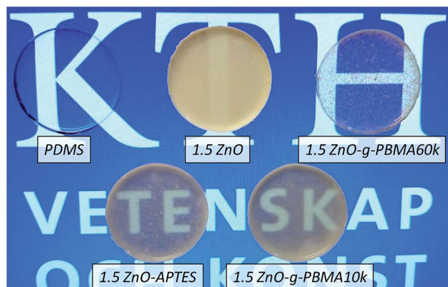
Fig. 7 Photo of neat PDMS and nanocomposites containing 1.5 vol% of ZnO NPs, ZnO-APTES, ZnO-g-PBMA10k or ZnO-g-PBMA60k.
