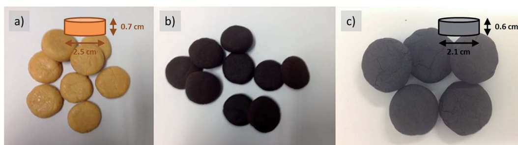
Fig. 4 Doughs obtained from glucose-urea-ZnCl 2 /H 2 O + 39% cellulose before and after baking (a) viscoelastic pellets of the dough, (b) pellets pre-baked at 100 °C for 3 hours, the green body, and (c) carbonaceous pellets made at 500 °C in nitrogen atmosphere.
