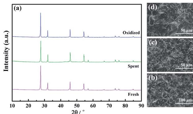
Fig. 11 The X-ray diffraction patterns (a) and SEM morphologies of fresh (b), spent (c) and oxidized (d)  $\text{La}_{5.5}\text{W}_{0.6}\text{Mo}_{0.4}\text{O}_{11.25-\delta}\text{F}_{0.05}$  membranes.
