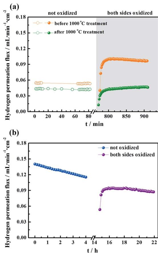
Fig. 10 (a) The regeneration of hydrogen permeation fluxes for the  $\text{La}_{5.5}\text{W}_{0.6}\text{Mo}_{0.4}\text{O}_{11.25-\delta}\text{F}_{0.05}$  membrane at  $950\text{ }^{\circ}\text{C}$ . (b) The oxidation effect on the permeability of the  $\text{La}_{5.5}\text{W}_{0.6}\text{Mo}_{0.4}\text{O}_{11.25-\delta}\text{F}_{0.05}$  membrane at  $1000\text{ }^{\circ}\text{C}$ .
