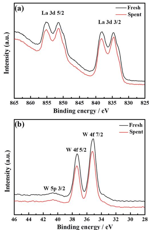
Fig. 8 La 3d (a) and W 4f (b) superimposed XPS spectra of fresh and spent La<sub>5.5</sub>W<sub>0.6</sub>Mo<sub>0.4</sub>O<sub>11.25-δ</sub>F<sub>0.05</sub> membranes.
