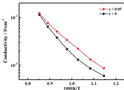
Fig. 6 Conductivity as a function of temperature plotted in the Arrhenius form under a wet ( $p_{\text{H}_2\text{O}} = 0.025$  atm) 10% hydrogen in argon atmosphere for  $\text{LWMF}_0$  and  $\text{LWMF}_{0.05}$  specimens.
