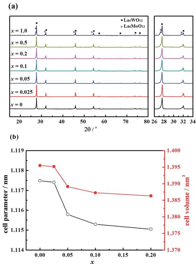
Fig. 1 (a) X-ray diffraction patterns and (b) the cell parameter and the cell volume of the  $\text{La}_{5.5}\text{W}_{0.6}\text{Mo}_{0.4}\text{O}_{11.25-\delta}\text{F}_x$  membranes sintered at  $1500^\circ\text{C}$ .
