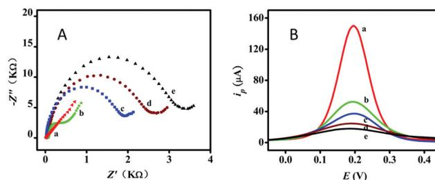
Fig. 2 EIS (A) and SWV (B) measurements of different electrodes in 0.4 M KCl containing 0.5 mM  $[\text{Fe}(\text{CN})_6]^{4-/3-}$  at the bare electrode (a), the capture DNA modified electrode (b), with MCH and BSA immobilized on the electrode surface (c), after hybridization with H1–H2 complexes with the target miRNA (d), and after RCA (e).
