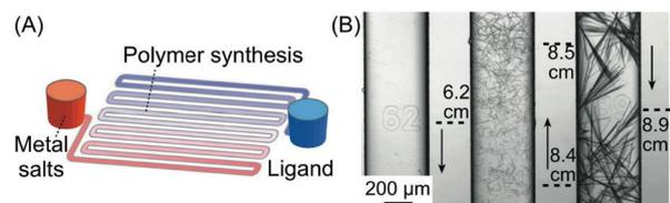
**Fig. 9** (A) Schematic illustration of the device used for the synthesis of silver acetylides. (B) Microphotographs showing the distribution and morphology of silver acetylide crystals formed along the microchannel. Adapted from ref. 31 with permission from Wiley-VCH Verlag GmbH & Co., copyright 2015.
