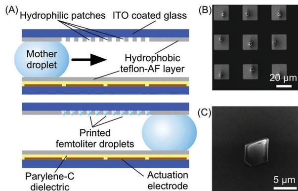
**Fig. 8** (A) Schematic illustration of the digital microfluidic device used in this experiment and of its functioning. (B) SEM image showing the array of HKUST-1 crystals fabricated by this technology. (C) Details of a single HKUST-1 crystal. Adapted from ref. 30 with permission from Wiley-VCH Verlag GmbH & Co., copyright 2012.
