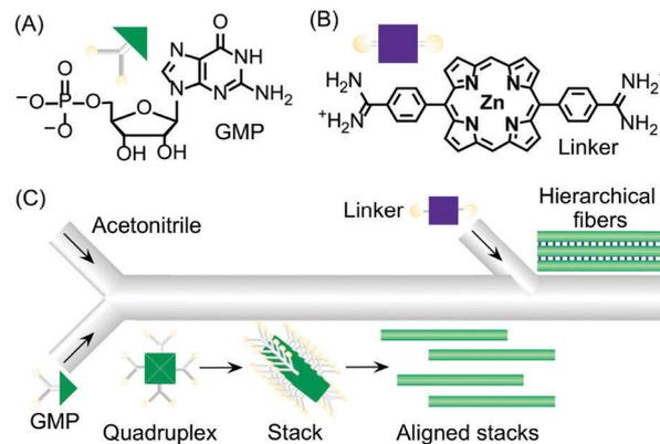
**Fig. 15** (A) Chemical structure of GMP. (B) Chemical structure of the bis-cationic linker porphyrin. (C) Schematic illustration of the microfluidic setup used in the experiment and of the hierarchical growth of GMP microfibrils by stepwise activation of non-covalent intermolecular interactions by spatial and temporal control. Adapted from ref. 38 with permission from Wiley-VCH Verlag GmbH & Co., copyright 2013.
