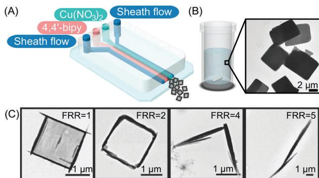
**Fig. 5** (A) Illustration of the microfluidic setup used in the experiments. (B and C) Transmission electron microscope (TEM) images of the CP synthesized in flask mixing experiments and with the continuous-flow microfluidic device at different FRRs, respectively. Adapted from ref. 24 with permission from Wiley-VCH Verlag GmbH & Co., copyright 2016.
