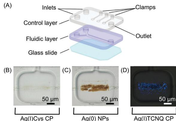
**Fig. 10** (A) Schematic view of the two-layer microfluidic platform employed in the study. (B–D) A sequence of optical microscope images showing the Ag(I)Cys CP assembled at the reactant interface; its reduction to Ag(0); and the subsequent formation of Ag(I)TCNQ (cross polarized image), respectively. Adapted from ref. 32 with permission from American Chemical Society, copyright 2014.
