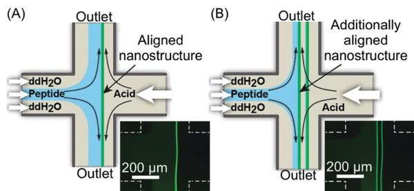
**Fig. 20** (A) Schematic illustration of the fluidic-directed synthesis of 1D peptide–OPV fibers by using planar extensional flow, and fluorescence microscopy micrograph showing the emitting fiber grown at the reactive interface. (B) Schematic illustration and micrograph showing the formation of two aligned fibers obtained by modulating the flow rates, *i.e.* changing the position of the reactive interface. Adapted from ref. 44 with permission from Wiley-VCH Verlag GmbH & Co., copyright 2013.
