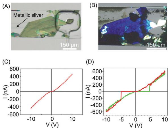
**Fig. 11** (A) Optical image of a large TCNQ crystal grown in the fluidic channel and trapped with a pneumatic clamp, and a line of generated silver metal. (B) Polarized optical image of the Ag(I) doped TCNQ crystal. The white areas correspond to the pure TCNQ, while the rest of the crystal shown is the Ag-TCNQ complex. (C)  $I/V$  sweep of the Ag(I)TCNQ complex and (D) of the intermediate region measured with CAFM. Adapted from ref. 33 with permission from The Royal Society of Chemistry.
