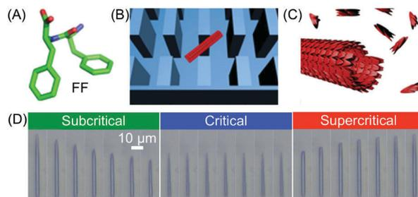
**Fig. 19** (A) Chemical structure of FF. (B) Schematic illustration of a single FF tube trapped between the micro-scale pillars. (C) Illustration of the FF nanotube growth. (D) Imaging of FF nanotubes at different times under subcritical (1.6 mM, 10 s interval), critical (2.43 mM, 60 s interval), and supercritical (3.20 mM, 100 s interval) concentration conditions. Adapted from ref. 42 with permission from Springer Nature, copyright 2016.
