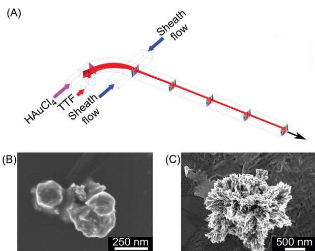
**Fig. 3** (A) Schematic drawing of the 3D hydrodynamic flow focusing device used for the shape control synthesis of TTF-Au structures. (B) and (C) SEM images of the structures collected at a FRR of 20 and 0.2, respectively. Adapted from ref. 22 with permission from American Chemical Society, copyright 2014.
