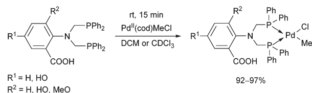
Scheme 24 Preparation of mononuclear Pd II complexes from \alpha -aminophosphines bearing a benzoic acid moiety.
