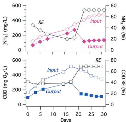
Fig. 7 NH<sub>3</sub> (top) and COD (bottom) averaged concentrations before (input) and after (output) an electrochemical treatment cycle of 4 hours with respective removal efficiencies (RE) for 30 continuous days of operation of YXG prototype. Day 0 corresponds to the beginning of usage of the prototype.
