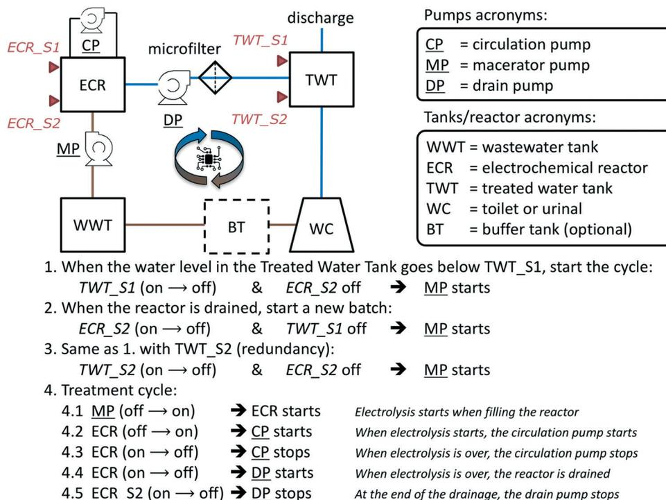
**Fig. 3** System flow diagram (top left, see Fig. S1† for volumes and residence times) with automation algorithm description for the onsite toilet wastewater treatment and recycling systems. Pumps are underlined. Capacitive level sensors are represented by red triangles. Brown lines illustrate the flow of untreated wastewater while blue lines illustrate the flow of treated and recycled wastewater.
