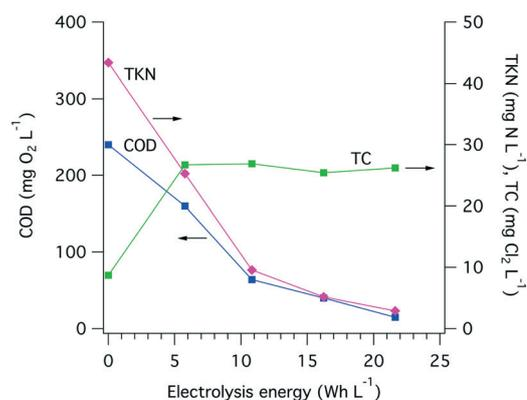
**Fig. 6** Evolution of the COD, TKN, and TC during the treatment of toilet wastewater in a single electrochemical treatment cycle in AMD prototype on 01/12/2015. Each point represent the average of three triplicate measurements.
