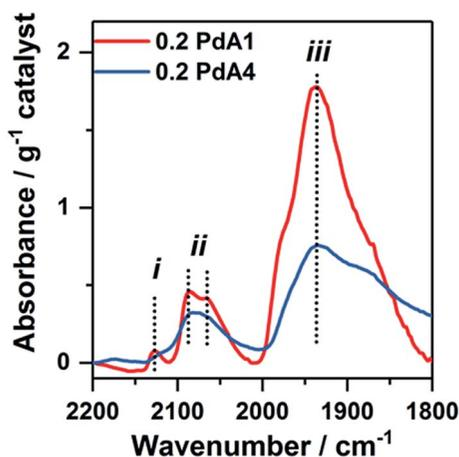
Fig. 3 FTIR spectra from CO-adsorption studies onto different 0.2 wt% Pd/TiO<sub>2</sub> catalysts: red = 0.2 PdA1 and blue = 0.2 PdA4.
