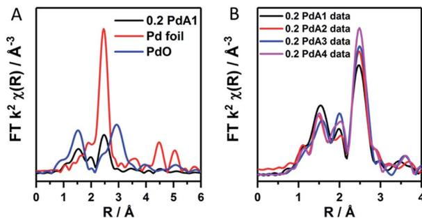
Fig. 2  $k^2$  weighted forward FT data for (A) the 0.2 PdA1 catalyst (1 °C  $\text{H}_2\text{O}$ ), Pd foil and PdO reference, and (B) all 0.2 wt% Pd/TiO<sub>2</sub> catalysts.
