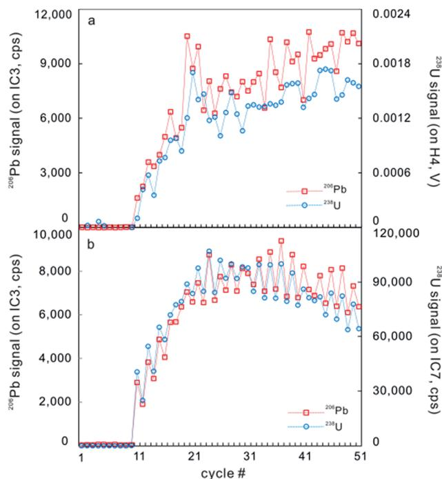
Fig. 5 A typical time-resolved profile on GJ-1 zircon for continuous laser ablation analysis measured on a Neptune Plus. (a) Signals of <sup>206</sup>Pb (red) and <sup>238</sup>U (blue) were counted on IC3 and Faraday cup H4, respectively. (b) Signals of <sup>206</sup>Pb (red) and <sup>238</sup>U (blue) were counted on IC3 and IC7, respectively (from ref. 5).
