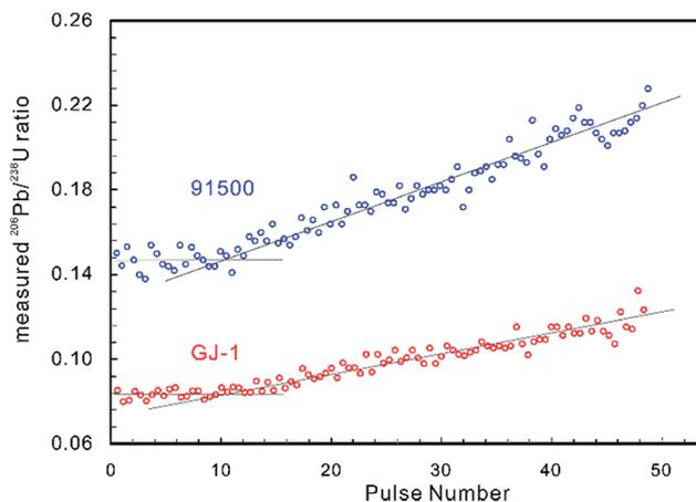
Fig. 2 The measured  $^{206}\text{Pb}/^{238}\text{U}$  ratios of zircon reference materials 91500 (in blue) and GJ-1 (in red) by LA-MIC-ICP-MS show that the ratio is stable to a depth of about 1.3  $\mu\text{m}$  (approx. 10 pulses and 130 nm per pulse) and then increases as the ablation continues (G2 laser ablation system at a laser fluence of 4  $\text{J cm}^{-2}$ , repetition rate of 4 Hz and beam size of 5  $\mu\text{m}$ ).
