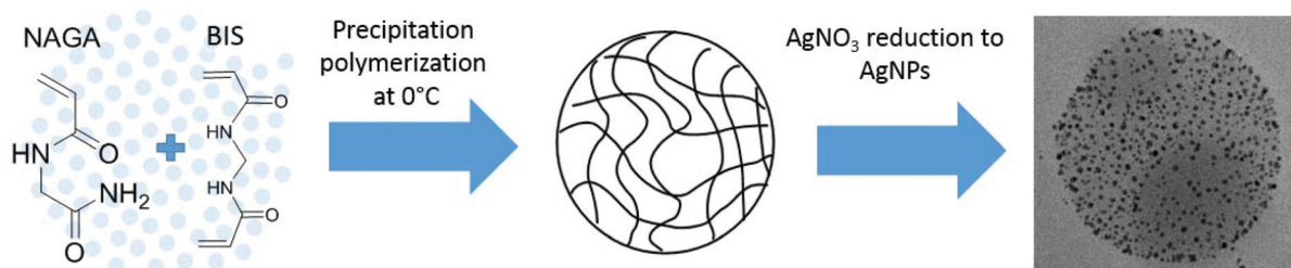
Scheme 1 Schematic illustration of the synthesis route to PNAGA microgels and Ag-PNAGA hybrid microgels.
