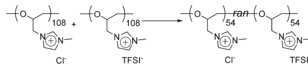
Scheme 2 Synthesis of poly(ECH-Melm ^+\text{Cl}^- - ran -ECH-Melm ^+\text{TFSI}^- ) just by mixing poly(ECH-Melm ^+\text{Cl}^- ) and poly(ECH-Melm ^+\text{TFSI}^- ).
