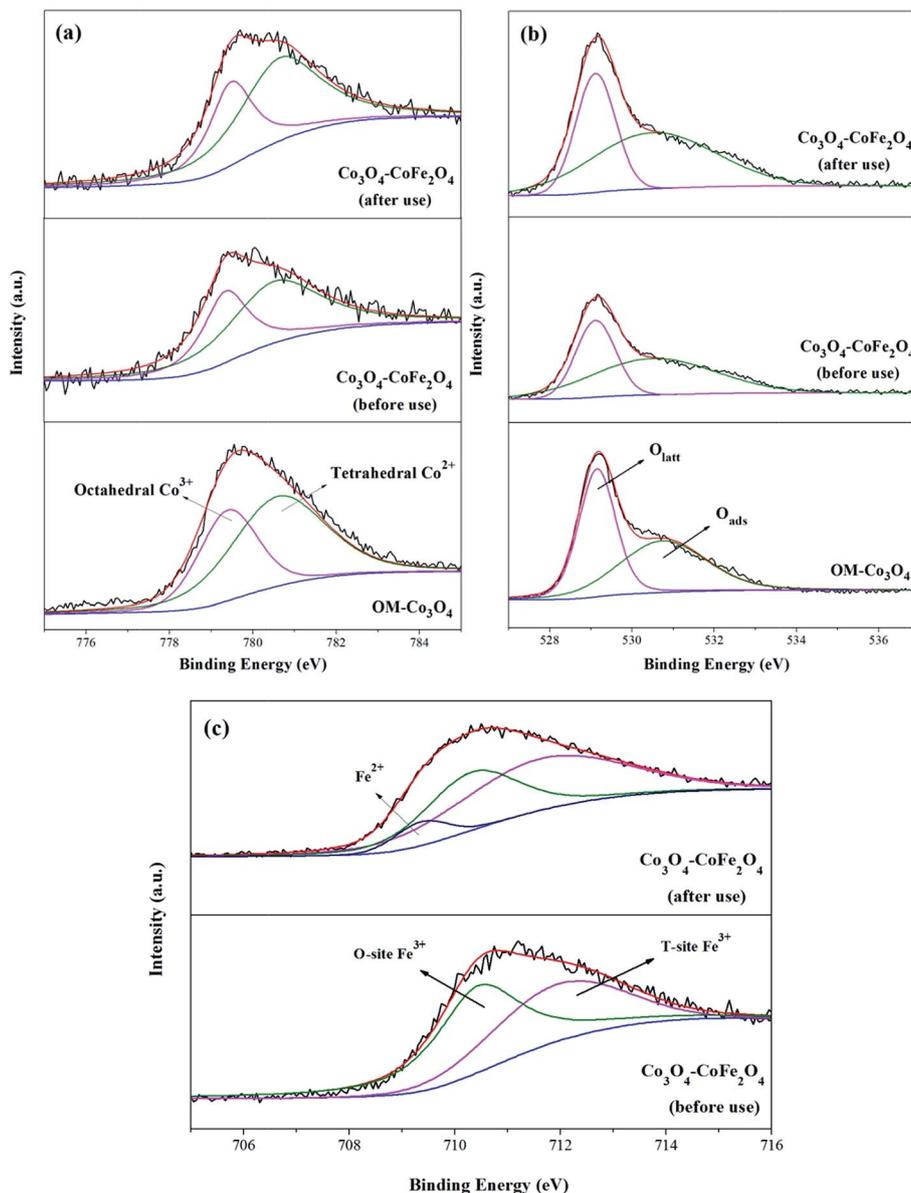
Fig. 4 XPS survey spectrum of Co 2p<sub>3/2</sub> (a), O 1s (b) and Fe 2p<sub>3/2</sub> (c) for OM-Co<sub>3</sub>O<sub>4</sub> and Co<sub>3</sub>O<sub>4</sub>-CoFe<sub>2</sub>O<sub>4</sub>.
