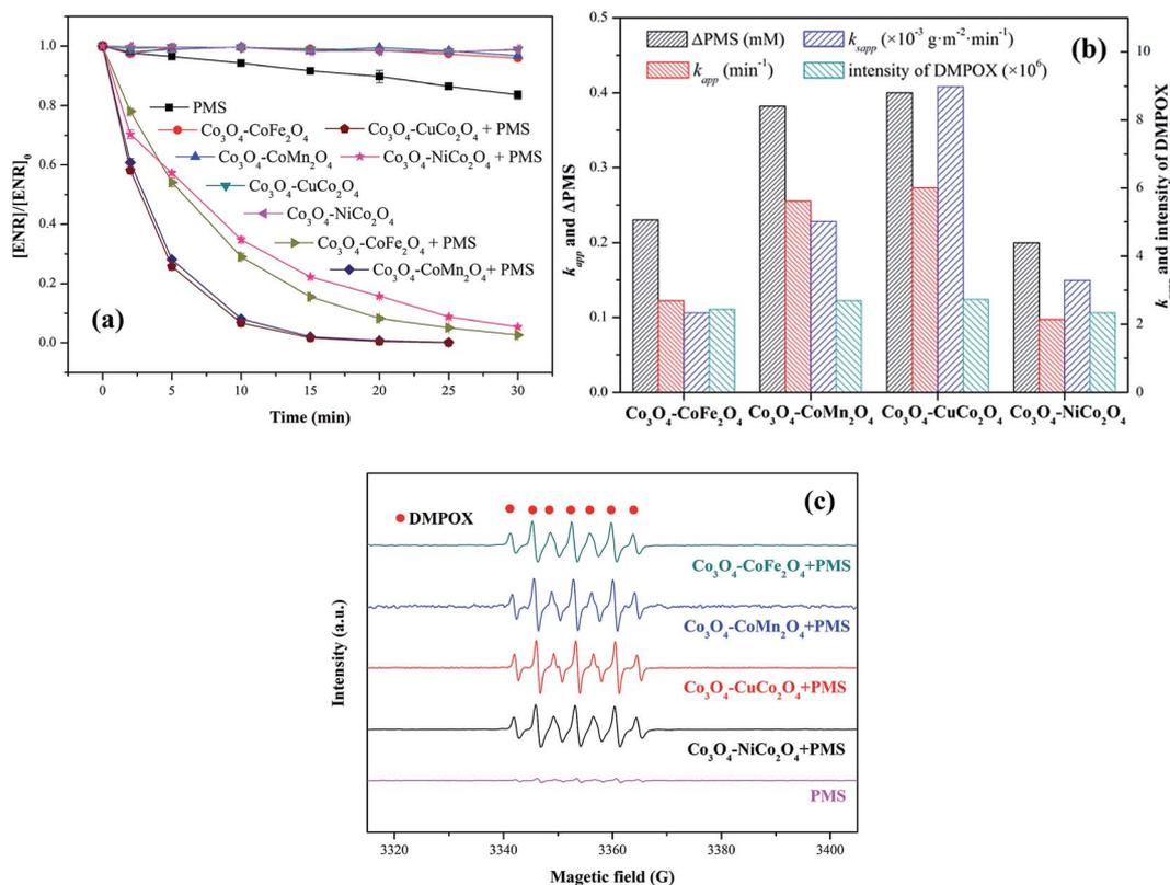
Fig. 5 (a) ENR degradation in different systems; (b) values involved in different Co<sub>3</sub>O<sub>4</sub>-composite spinels/PMS systems; (c) EPR spectra in different composite spinels/PMS systems (DMPO = 25 mM). Experimental condition: [ENR] = 10 mg L<sup>-1</sup>, [catalyst] = 0.1 g L<sup>-1</sup>, [PMS] = 1 mM, pH<sub>0</sub> = 6, T = 25 °C.
