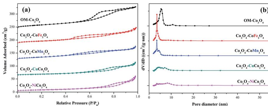
Fig. 3 (a) Nitrogen adsorption–desorption isotherms of OM- $\text{Co}_3\text{O}_4$  and  $\text{Co}_3\text{O}_4$ -composite spinels and (b) their pore size distributions.
