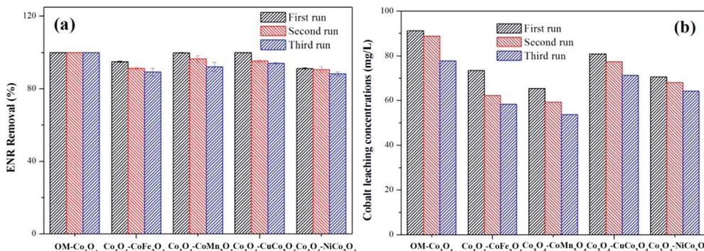
Fig. 9 (a) Reusability of different  $\text{Co}_3\text{O}_4$ -composite spinels as catalyst for the degradation of ENR; (b) cobalt leaching concentrations in different  $\text{Co}_3\text{O}_4$ -composite spinels/PMS systems. Experimental condition:  $[\text{ENR}] = 10 \text{ mg L}^{-1}$ ,  $[\text{catalyst}] = 0.1 \text{ g L}^{-1}$ ,  $[\text{PMS}] = 1 \text{ mM}$ ,  $\text{pH}_0 = 6$ ,  $T = 25 \text{ }^\circ\text{C}$ , reaction time = 25 min.
