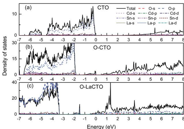
Fig. 3 Total and partial density of states of (a) perfect  $\text{Cd}_2\text{SnO}_4$  and (b) the  $\text{V}_{\text{O}_2}$  oxygen vacancy of  $\text{Cd}_2\text{SnO}_4$  and (c) La-doped  $\text{Cd}_2\text{SnO}_4$  based on the  $\text{V}_{\text{O}_2}$  oxygen vacancy, respectively.
