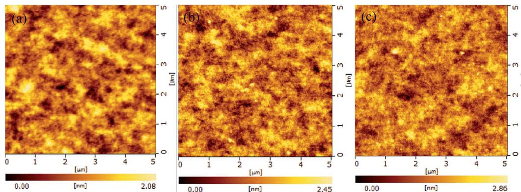
Fig. 5 The AFM morphologies of the conjugated polymers HPF-Ir10, LPF-Ir10 and ELPF-Ir5 films coated on the ITO glasses (5 × 5 μm<sup>2</sup>).
