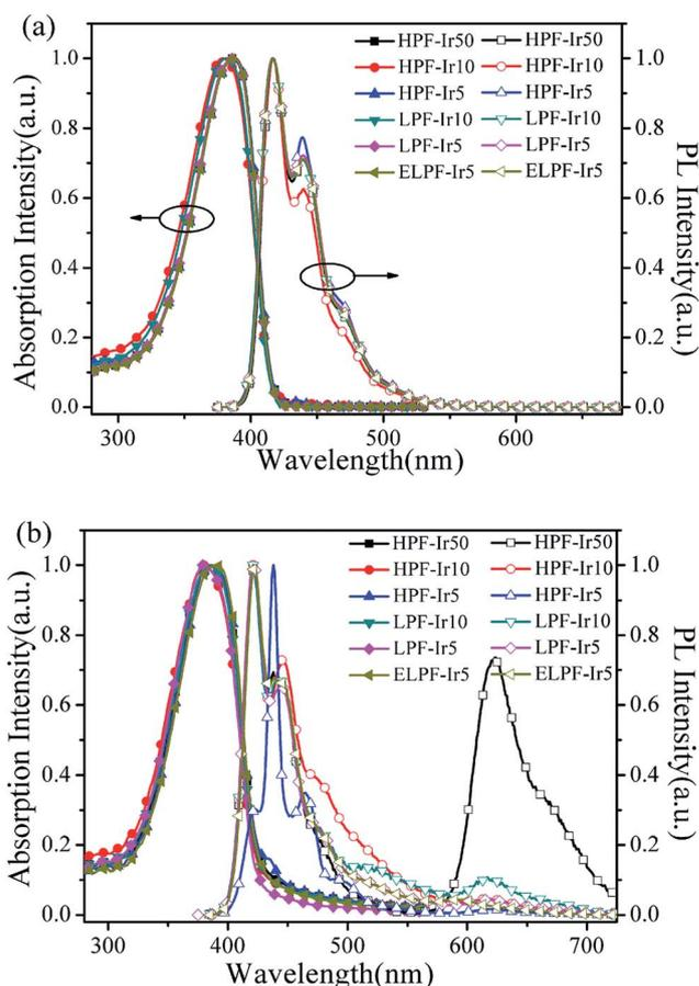
Fig. 1 UV-vis spectra and PL spectra of the conjugated polymers in CHCl<sub>3</sub> solution (a) and films (b).
