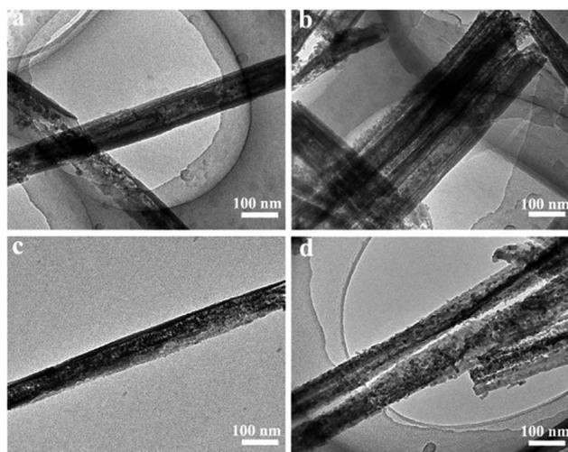
Fig. 1 TEM images of halloysite nanotubes after being etched by HCl at 80 °C for (a) 6 h, (b) 7.5 h, (c) 11 h and (d) 18 h, respectively.
