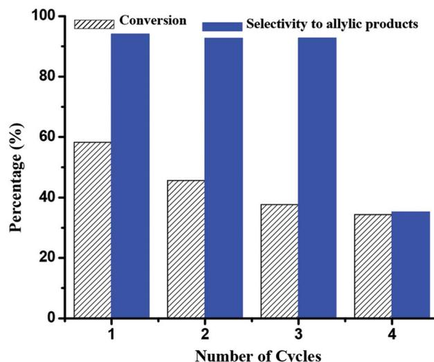
Fig. 6 The cycling stability of cyclohexene oxidation with HA/HCl-18 h/Co<sup>2+</sup>-2 : 1 as catalyst.
