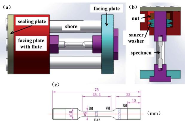
Fig. 2 Schematic diagrams of: (a) overall view of the assembly, (b) sectional view of self-loaded frame and specimen, and (c) dimensions of specimen.
