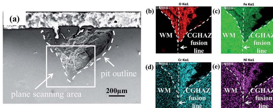
Fig. 14 (a) SEM image of a corrosion pit formed in a welded joint for the immersion time of 1254 hours under the action of a tensile stress of  $0.3\sigma_y$ ; EDS maps of elements near the corrosion pit: (b) O element, (c) Fe element, (d) Cr element, and (e) Ni element.
