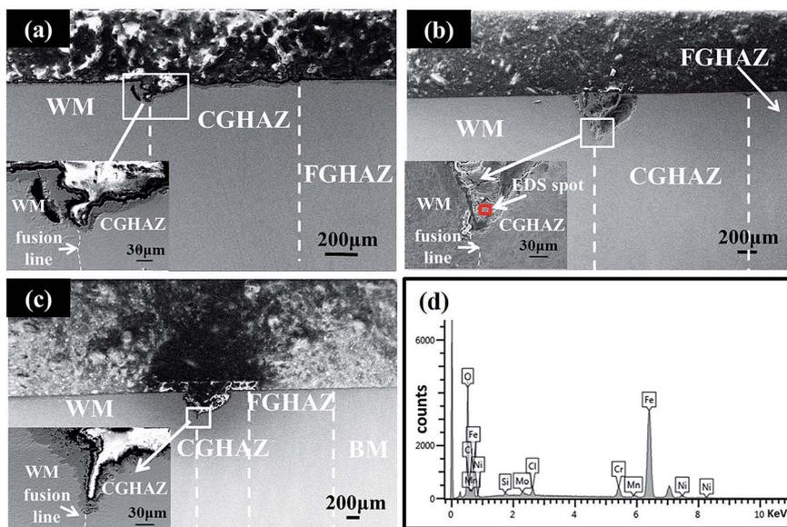
Fig. 6 SEM images of the cross section surface of the corroded joints under the action of different tensile stresses at different immersion times; (a)  $\sigma = 0$ , time = 1254 hours, (b)  $\sigma = 0.3\sigma_y$ , time = 1254 hours, and (c)  $\sigma = 0.9\sigma_y$ , time = 1080 hours; (d) EDS of the corrosion products shown in (b).
