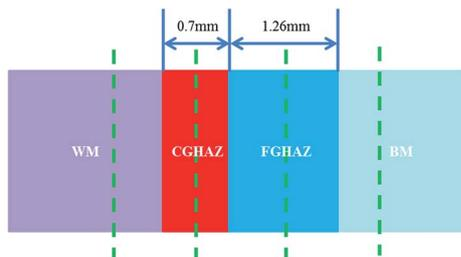
Fig. 1 Schematic diagram showing that the specimen location in the different regions of welded joint used in the electrochemical measurement (CGHAZ: coarse-grained HAZ, FGHAZ: fine-grained HAZ).
